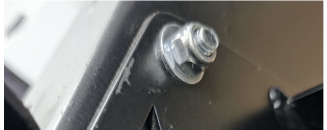
SMALL WASHER + NYLOC NUT - INSIDE
