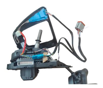
The single white/black wire near the 12 way Deutsch connector is grounded when the shifter is in park. This could be utilised if you wanted to fit a park start inhibit.
