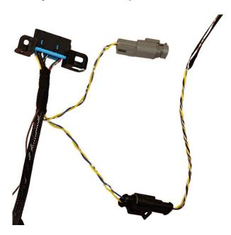
As with all CANBus circuits, the resistance between CAN High and CAN Low must be 60 ohms.
