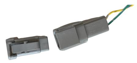
We recommend checking the CANBus resistance with a multimeter before connecting the plug in resistor.
