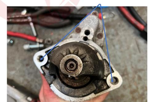
Once the starter has been fitted, the adapter plate should now be installed onto the engine. If your engine block already has dowels fitted in the outer 2 holes, carefully line the adapter up and push it into place. Note: a tap with a small rubber mallet may be required to correctly seat the plate on the dowels.
