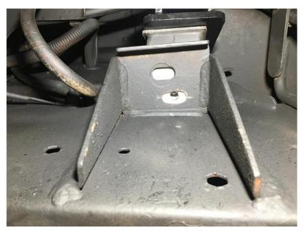
Fit the rubber mount to the mounting bracket and then secure mounting bracket through the left-hand holes of the House of Torque BMW6/8hp-LT230 Adapter Plate as pictured. (Threads from these holes may require removal with 10.5mm drill bit).
