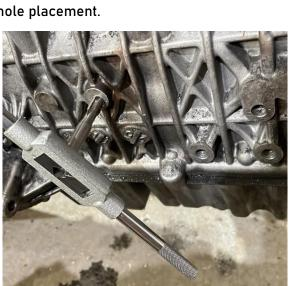
8.5mm an M10 tap can be used to make the thread.
