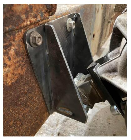
The original 300tdi transfer box mount can be reused with the new rubber supplied. Torque the M12 bolts to 100nm and M10 nyloc nuts to 55nm.
