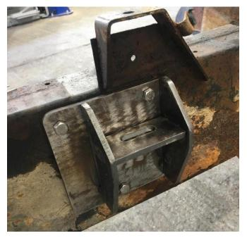
Fit the rubber mount to the mounting bracket and then secure mounting bracket through the left-hand holes of the House of Torque BMW6/8hp-LT230 Adapter Plate. (Threads from these holes may require removal with 10.5mm drill bit).
