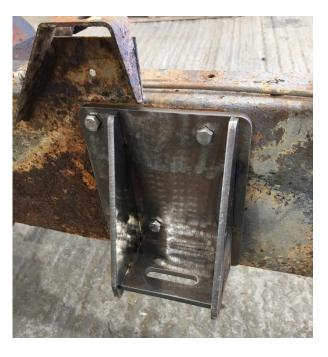
Replace the standard Land Rover transfer box mount with the unit supplied. Torque the M12 bolts to 100nm.
