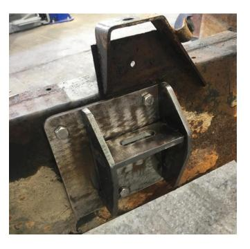
Fit the rubber mount to the mounting bracket and then secure mounting bracket through the left-hand holes of the House of Torque BMW6/8hp-LT230 Adapter Plate. (Threads from these holes may require removal with 10.5mm drill bit).
