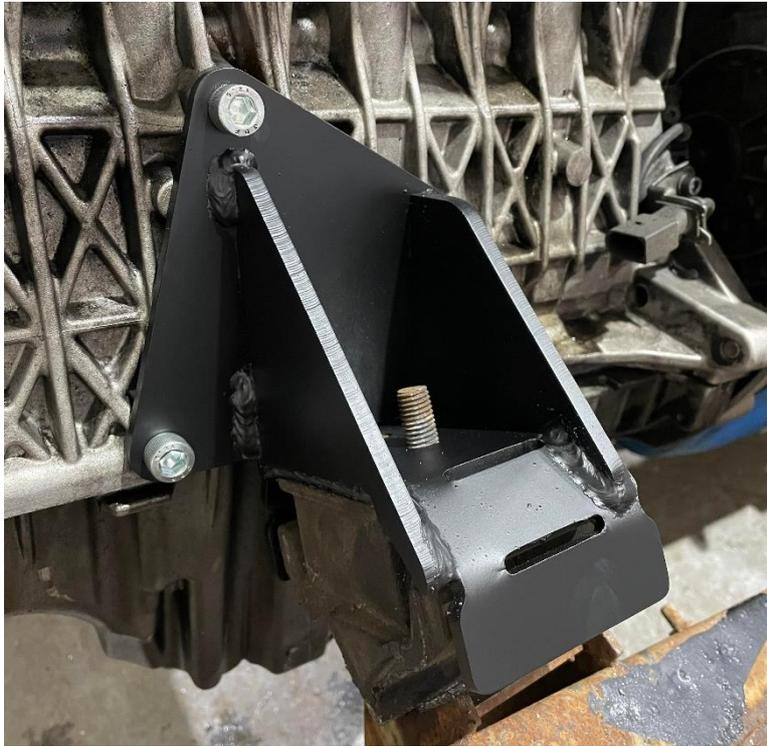
Elongate or drill an additional mounting hole for the engine mount rubber on the left hand chassis bracket as shown below.
