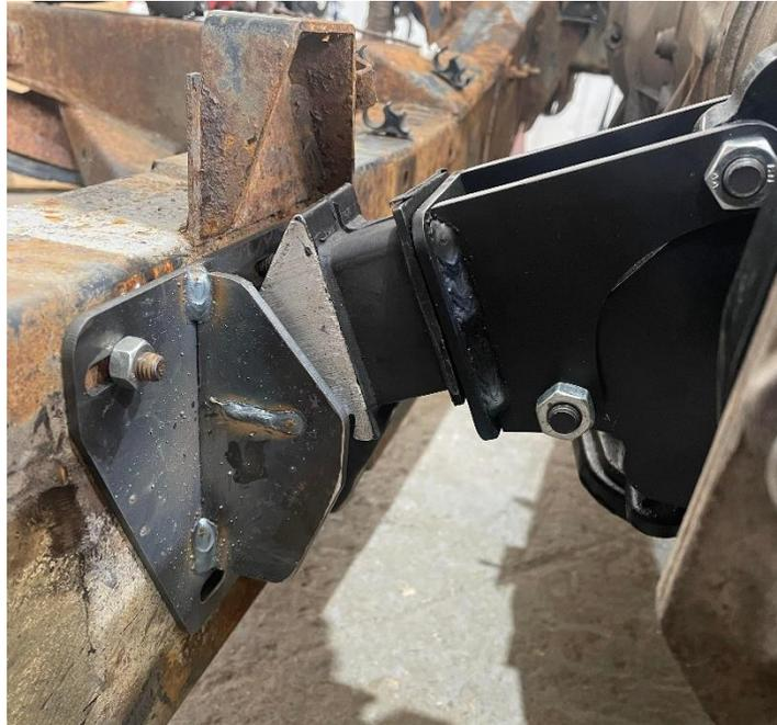
Fit the rubber mount to the mounting bracket and then secure mounting bracket through the left-hand holes of the House of Torque BMW6/8hp-LT230 Adapter Plate as pictured. (Threads from these holes may require removal with 10.5mm drill bit).
